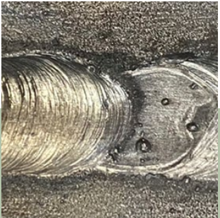
Initial situation: Insufficiently filled end crater
