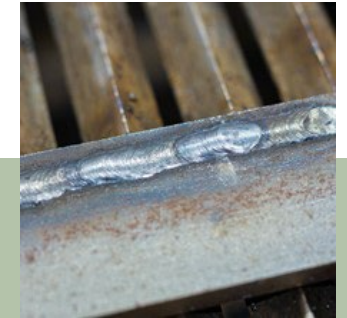
Brush rewelded zone → Result: Completely filled end crater and perfect overlap
