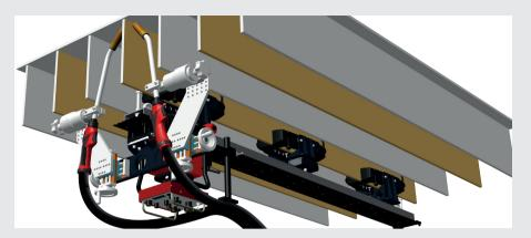
/ Extension for 2<sup>nd</sup> torch / Manual torch positioning in horizontal and vertical direction
