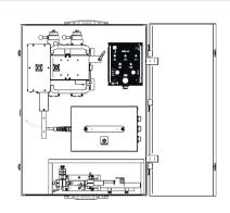
/ Custom fitting metal transport box including a toolkit for the entire system (rails separately).
