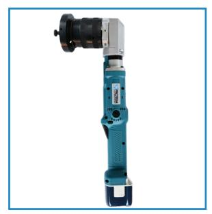
The OD Mounted Facing machine SE65RA clamps on the outside Ø of the tube with clamping collets. One collet per Ø is necessary. No distortion of the tubes, even for the thinnest ones.
