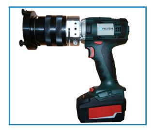
The OD Mounted Facing machine SE65 clamps on the outside  $\emptyset$  of the tube with clamping collets. One collet per  $\emptyset$  is necessary. No distortion of the tubes, even for the thinnest ones.
