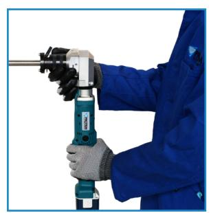
The OD Mounted Facing machine SE25RA clamps on the outside  $\emptyset$  of the tube with clamping collets. One collet per  $\emptyset$  is necessary. No distortion of the tubes, even for the thinnest ones.
