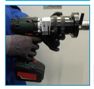
The OD Mounted Facing machine SE25 clamps on the outside  $\emptyset$  of the tube with clamping collets. One collet per  $\emptyset$  is necessary.
