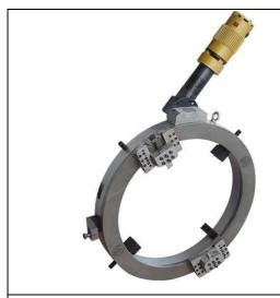
Working range: 600-750mm Cutting thickness: 5-25mm Rotational speed: 7r/min
