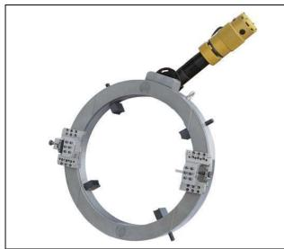
Working range: 450-600mm Cutting thickness: 4-25mm Rotational speed: 8r/min
