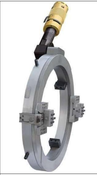
Working range: 900-1050mm Cutting thickness: 6-25mm Rotational speed: 5r/min
