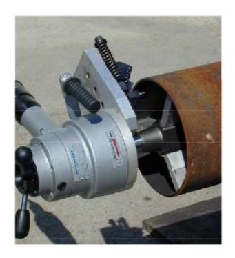
The option enables bevelling the oval pipes with retaining the uniform phase
