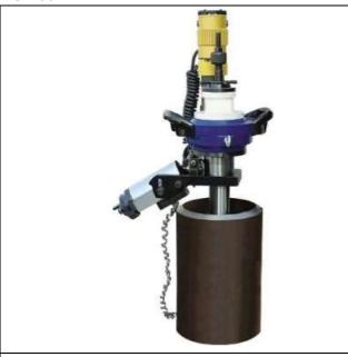
Working Range: 150-352mm Cutting thickness: 15-75 mm
