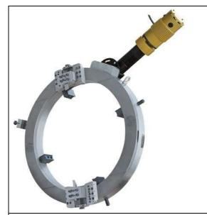
Working Range: 750-900mm Cutting thickness: 6-25mm Rotational speed: 6r/min
