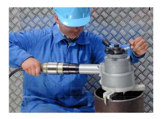
PRO10-PB pipe bevelling machine issigned for portable use on pipe machining operations. It allows efficient use by single operator. It is a typical heavy duty ID mounting pe be veler. PRO10-PB is able to bevel, face off and counterbore simultaneously in separate operations.
