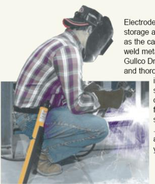
Electrode moisture absorption between oven storage and welding has long been recognized as the cause of high levels of hydrogen in the weld metal and costly weld rejects/failures. The Gullco Dry Pack provides an effective, affordable and thoroughly proven solution to this problem
