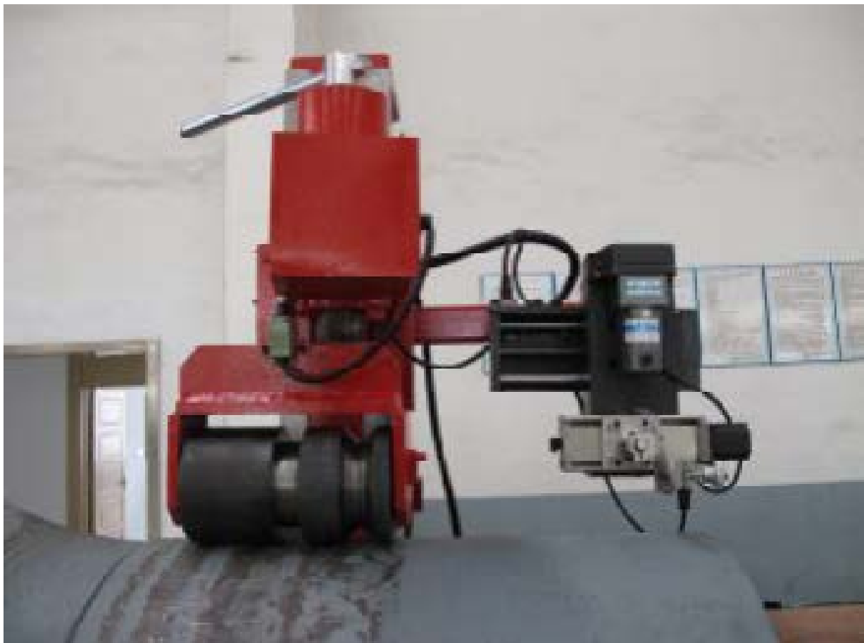
Torch bracket and oscillator (tonch screen is mounted on the control pendant)
