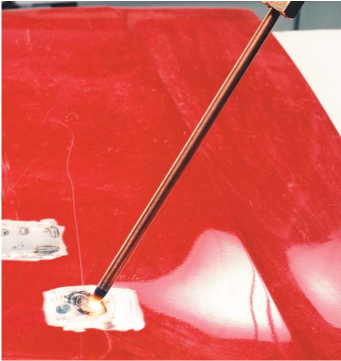
• Carbon arc electrode for heat shrinking
