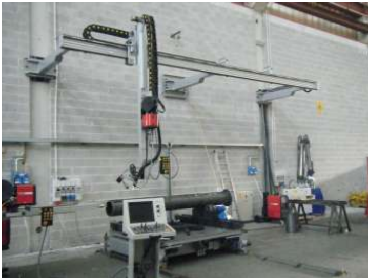
APTMMIDI Aluminum beam 120 x170 mm V - Steel guide 55 x25 mm
