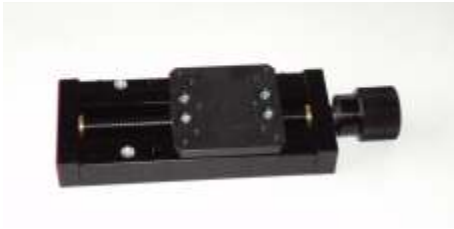
SMMD80-1 Slide with an axis, effective stroke 80 mm, with the follow features: Structure in machined aluminum, trapezoidal brass screw with nut, brass carriage guide and dovetail with gib for the adjustment, handle in knurled aluminum.
